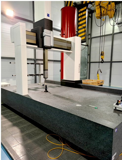
Рис. 5. Внешний вид КИМ Zeiss Accura 12/30/10 Fig. 5. Appearance of the Zeiss Accura coordinate measuring machine 12/30/10
